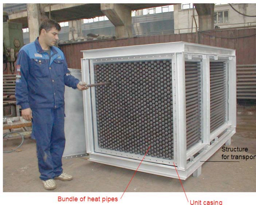
Figure 1 - Econotherm® GA units can be easily cleaned by simple pipe removal
